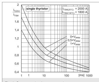
Fig. 8: Surge overload current vs. time
