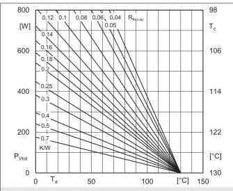
Fig. 4R: Power dissipation per module vs. ambient temperature
