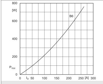
Fig. 4L: Power dissipation per module vs. direct current
