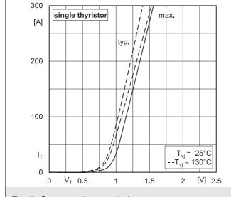
Fig. 7: On-state characteristics
