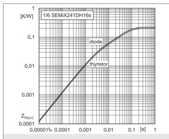
Fig. 6: Transient thermal impedance vs. time
